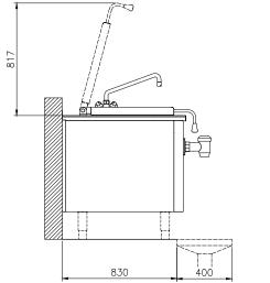
CWI1 = Cold Water inlet 1 (cleaning) Electrical inlet (power) HWI Hot water inlet
